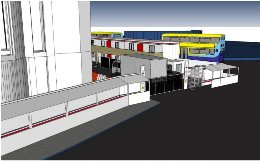
Figure 5. Example of Typical Hoarding
